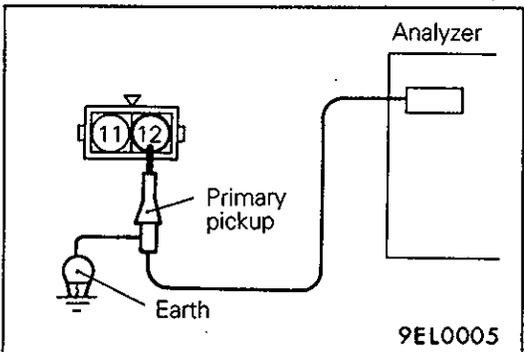
(2) Connect the analyzer primary pickup to the distributor connector terminal 12 .
