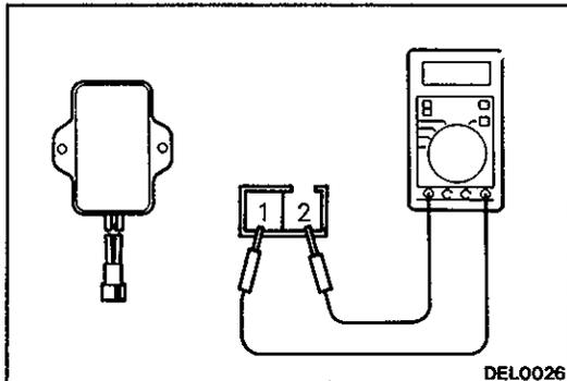
(2) Measure the resistance between the dropping resistor terminals.
