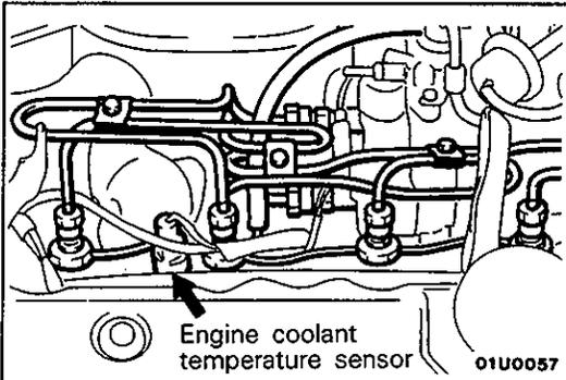
**ENGINE COOLANT TEMPERATURE SENSOR INSPECTION**
