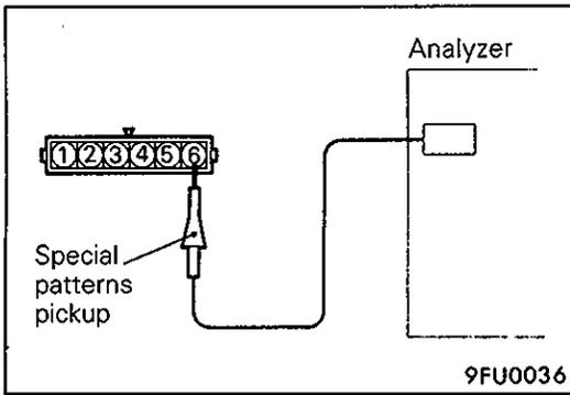
**Wave Pattern Inspection Using an Analyzer**
