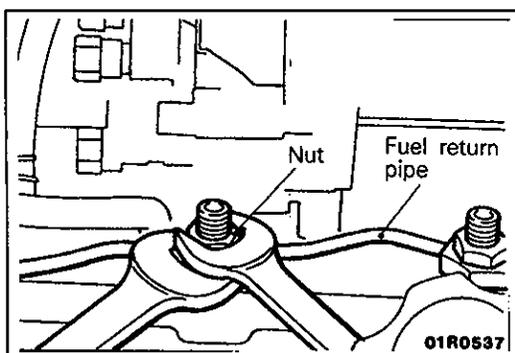
**17./18. REMOVAL OF NUT AND FUEL RETURN PIPE**
