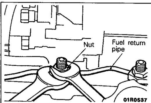
**18./17. INSTALLATION OF FUEL RETURN PIPE AND NUT**
