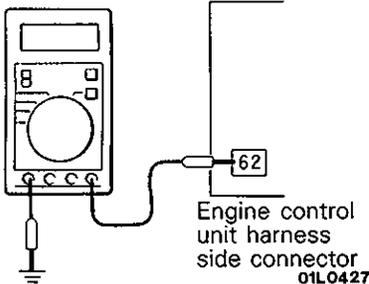
Engine control unit harness side connector
