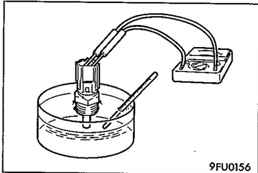
(2) With temperature sensing portion of coolant temperature sensor immersed in hot water, check resistance.
