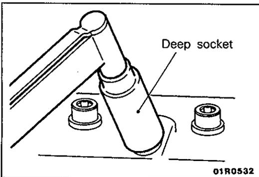
**20. INSTALLATION OF FUEL INJECTION NOZZLE**
