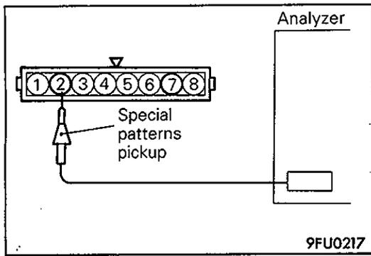
**Wave Pattern Inspection Using an Analyzer**
