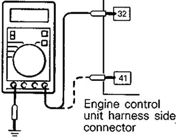
Engine control unit harness side connector
