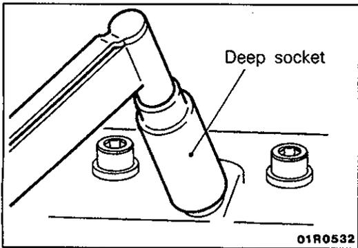
**20. REMOVAL OF FUEL INJECTION NOZZLE**
