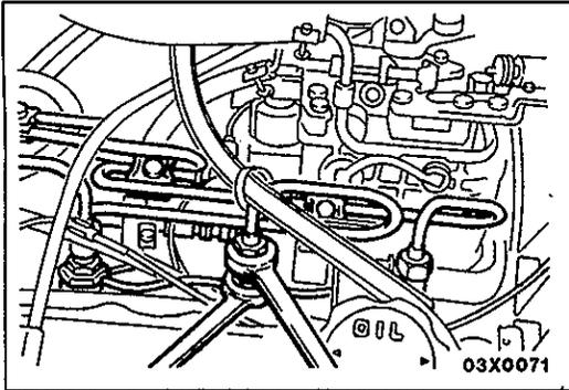
**SERVICE POINTS OF REMOVAL****7. REMOVAL OF FUEL INJECTION PIPE**
