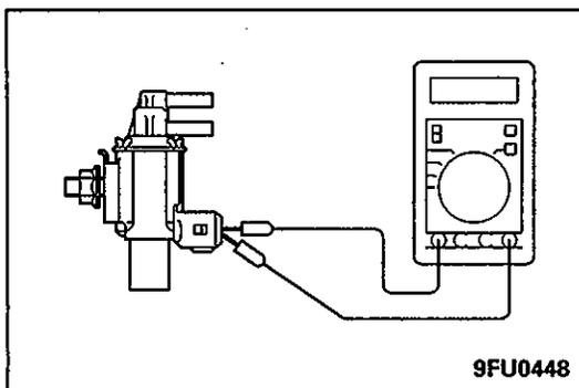
**INSPECTION OF AIR BY-PASS CONTROL SOLENOID VALVE COIL RESISTANCE**
