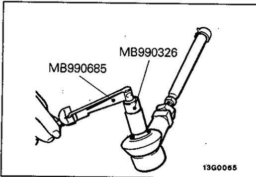
2. Move ball joint stud several times and install nut on stud. Measure ball joint starting torque with special tools.
