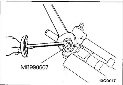
● **ADJUSTMENT OF TOTAL PINION PRELOAD**
