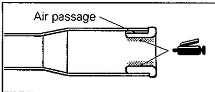
Caution: Take care that the applied grease does not obstruct the air passage of the rack bushing.
