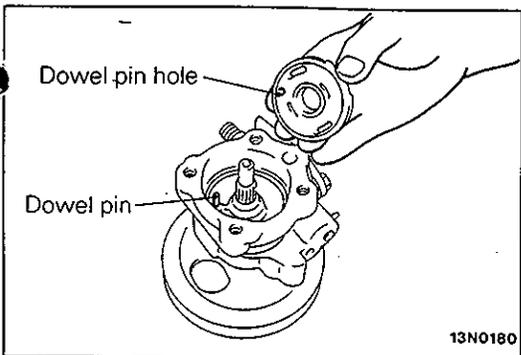
**6. INSTALLATION OF ROTOR**
