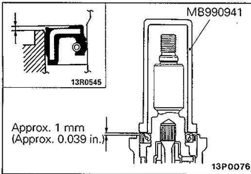
**18. INSTALLATION OF OIL SEAL**
