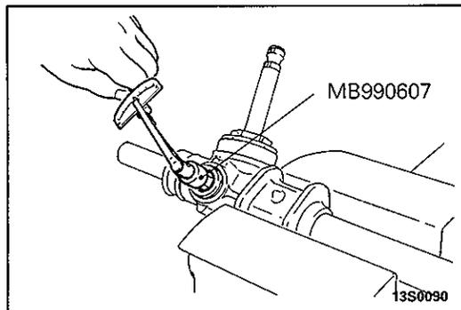
● **ADJUSTMENT OF TOTAL PINION PRELOAD**
