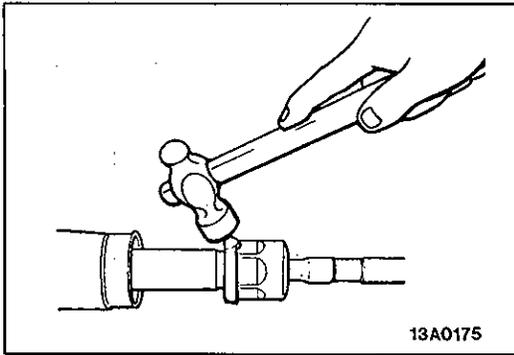
**10. INSTALLATION OF TAB WASHER/9. TIE ROD**
