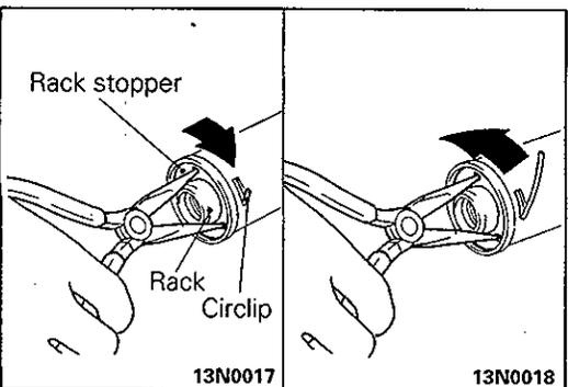
**24. REMOVAL OF CIRCLIP**
