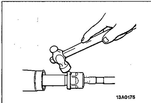
**8. INSTALLATION OF TAB WASHER/7. TIE-ROD**
