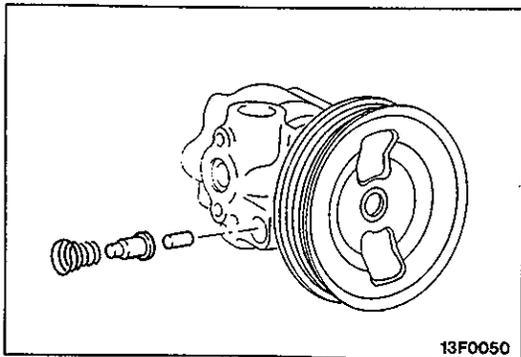
**8. INSTALLATION OF SIDE PLATE**
