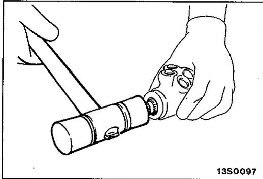
**18. REMOVAL OF OIL SEAL/19. PINION AND VALVE ASSEMBLY**
