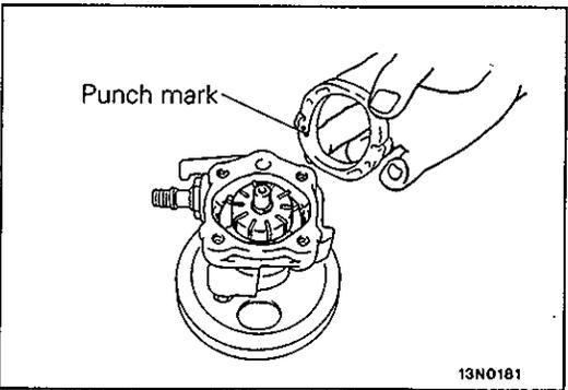
**4. INSTALLATION OF CAM RING**
