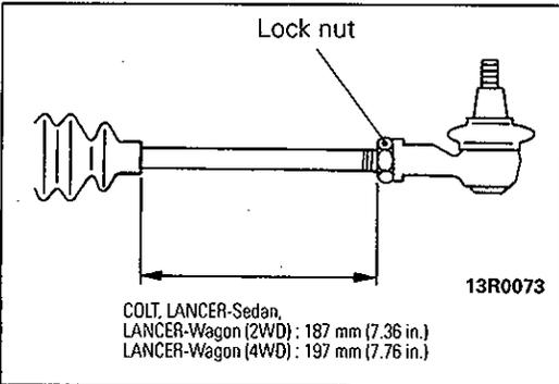
**4. INSTALLATION OF TIE ROD END/3. TIE ROD END LOCKING NUT**
