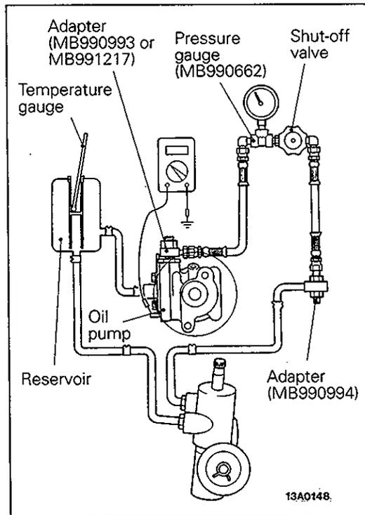
**POWER STEERING OIL PRESSURE SWITCH CHECK**
