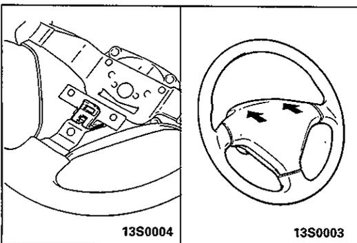
**4. INSTALLATION OF SPRING HOLDER/1. HORN PAD**
