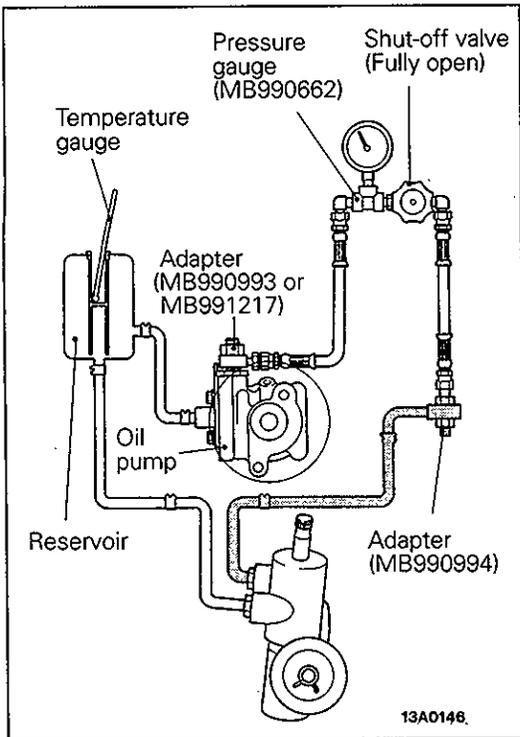
**CHECKING THE STEERING GEAR RETENTION HYDRAULIC PRESSURE**
