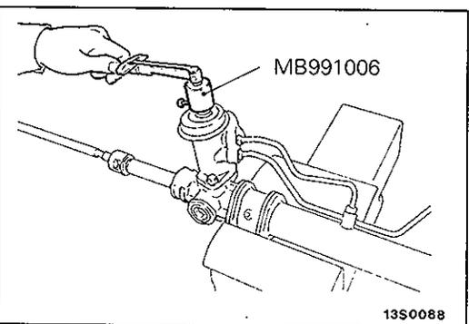
(3) Using the special tool, rotate the pinion gear at the rate of one rotation in approximately 4 to 6 seconds to check the total pinion preload.
