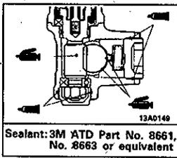
Sealant: 3M ATD Part No. 8661, No. 8663 or equivalent
